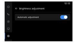
Turning on the automatic brightness adjustment, the brightness can adjusts automatically.
